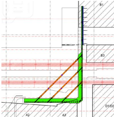
Plan view of L-shaped secant wall and temporary ties across the dock
